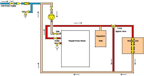
**Typical Mechanical Heating Installation**
